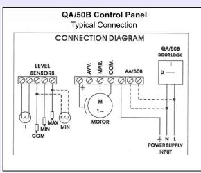
NB: To ensure a fully reliable low-level operation it is important to keep the probe rods free of debris. Anything that will prevent the passes between the conductive probes in the liquid could prevent the pump from starting or stopping at the desired water levels. Always check these periodically.
